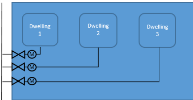
2. Multiple meters - (acceptable) to multiple units as long as there is one meter for every unit.
