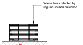
Waste Bin Area Elevation 4 1 : 100
